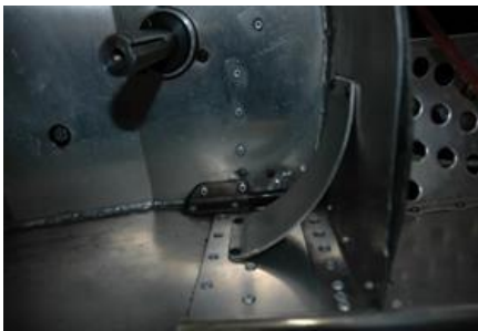
BELT GUARD WITH TOE PROTECTION DEVICE
