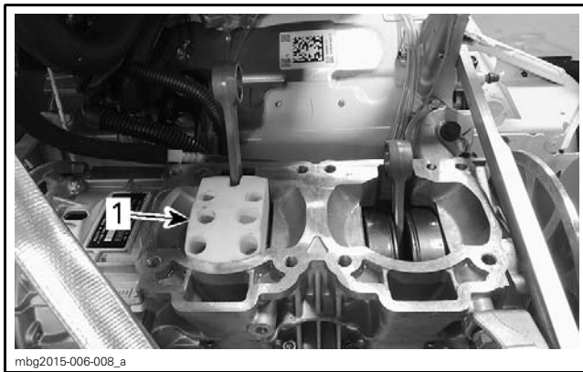
1. Crankshaft drilling guide
