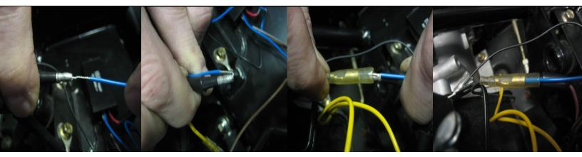
REV LIMITER WIRES CAN BE INSTALLED 2 DIFFERENT WAYS, 1 BY HARD-WIRING OR 2 USING THE METHOD ABOVE.
