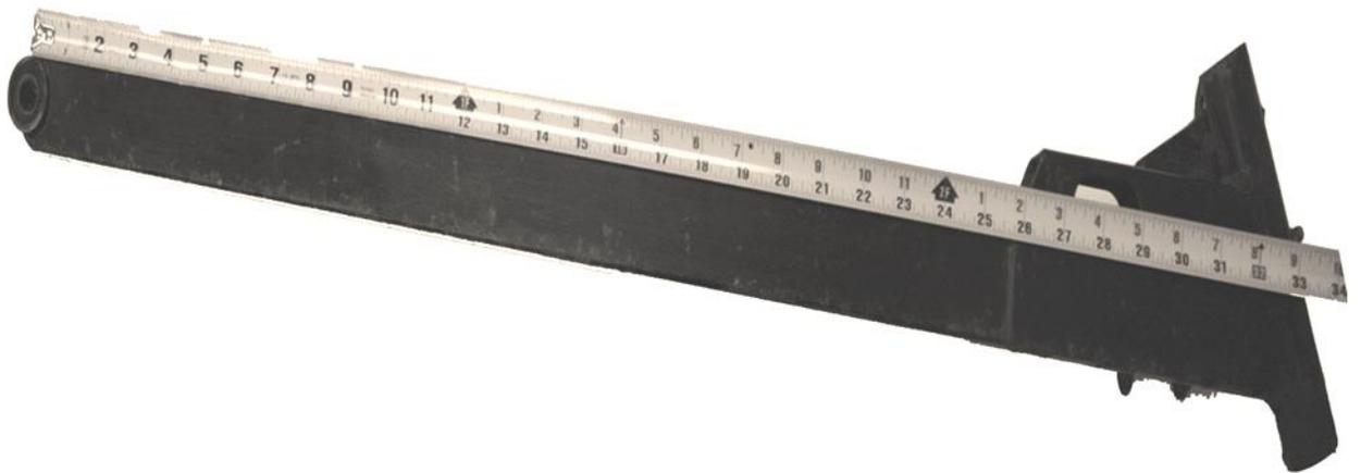
**Dimension is from center line on rear trailing arm mount, to reference mark or grease zerk depending on if using OEM or aftermarket trailing arm. The length required is 33 inches.**
